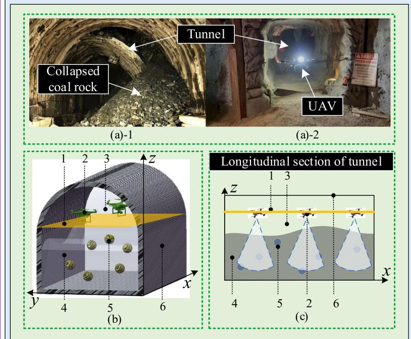
The electromagnetic target is covered by rock and coal following the tunnel accident in the coal mine, and the UAV searches the accident site for the electromagnetic target. The residual electromagnetic target is located and connected to enable the establishment of an emergency communication network in the accident site.
