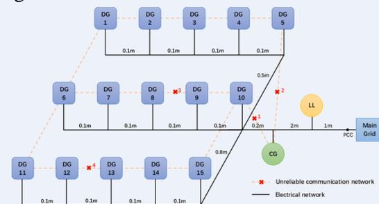
Fig. 2. Microgrid system considered in simulation.
