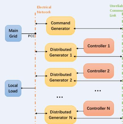
Fig. 1. Grid-connected Microgrid.
