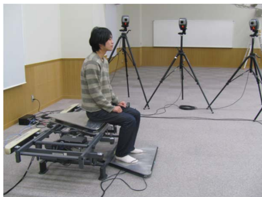
Measurement system for standing-up motion (Motion Capture and force measurement)
