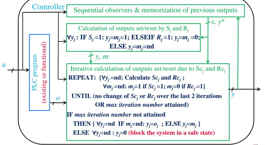
Converges if number of iterations ≤ twice the number of outputs with combined functions, otherwise the system is blocked in a safe state if constraints are badly defined or if a malfunction occurs
