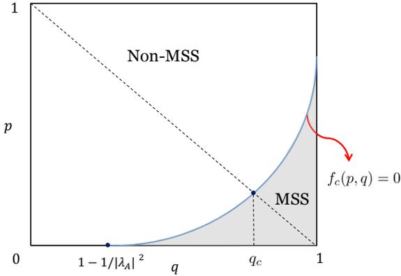
Fig. 2: The  $p - q$  plane is divided into MSS (Mean-square Stability) and Non-MSS regions by the critical curve  $f_c(p, q) = 0$ . When  $p + q = 1$ , the Markovian packet loss process is reduced to an i.i.d. process. As a result, the intersection point of the curves  $f_c(p, q) = 0$  and  $p + q = 1$  gives the critical packet drop probability established in [9].
