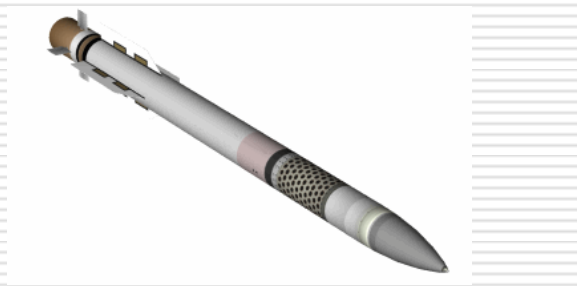
Compound control: lateral jets and aerodynamic fins
